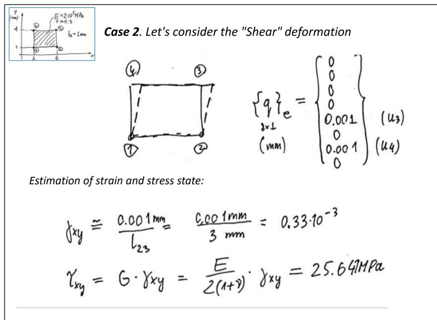
Let's calculate the strains in the element from the strain-displacement matrix:
