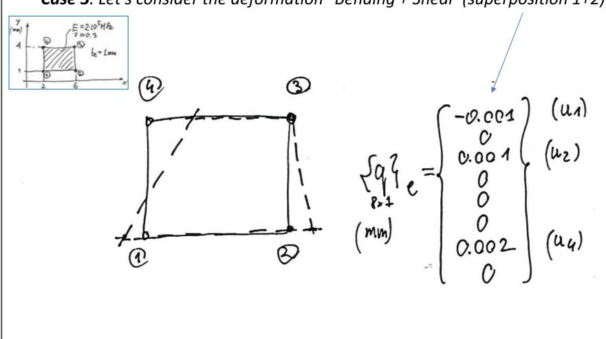
**Case 3**. Let's consider the deformation "Bending + Shear" (superposition 1+2)
