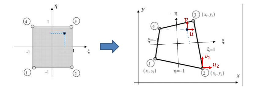
Geometry mapping:  $(\xi, \eta) \to (x, y)$  $(-1, -1) \to (x_1, y_1)$   $(1, -1) \to (x_2, y_2)$   $(1, 1) \to (x_3, y_3)$   $(-1, 1) \to (x_4, y_4)$
