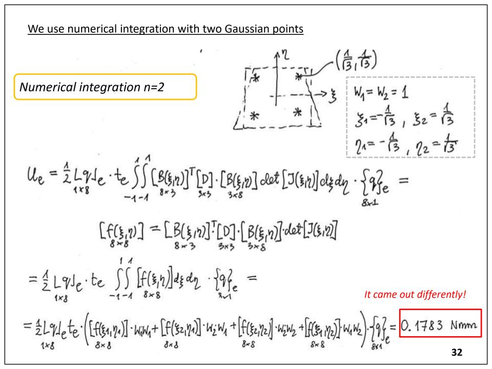
Let's try to calculate the elastic strain energy of the element again differently (separately for normal stress and separately for shear stress):
