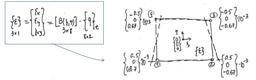
We will calculate the components of the stress state using the matrix of elastic constants:
